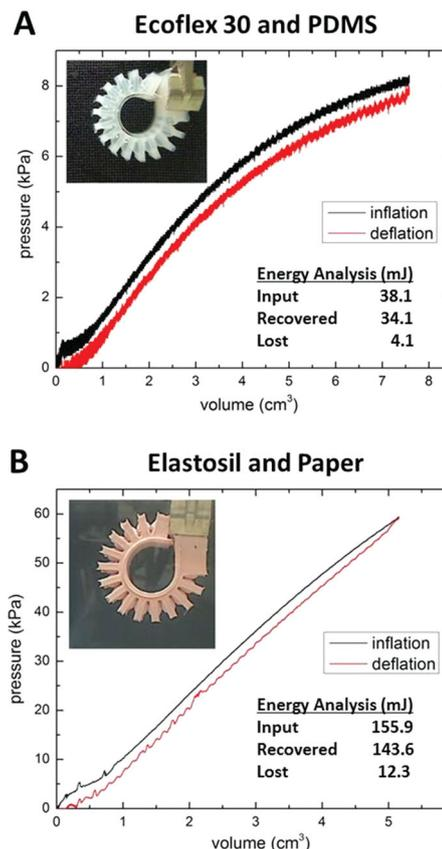
**Figure 3.** Effect of Elastomer Stiffness. A,B) Pressure–volume hysteresis curves for fPN actuators fabricated with an extensible layer made from Ecoflex 30 and an inextensible layer made from PDMS (A) and an extensible layer made from Elastosil M4601 and inextensible layer made from a composite of Elastosil M4601 and paper fabric (B).
