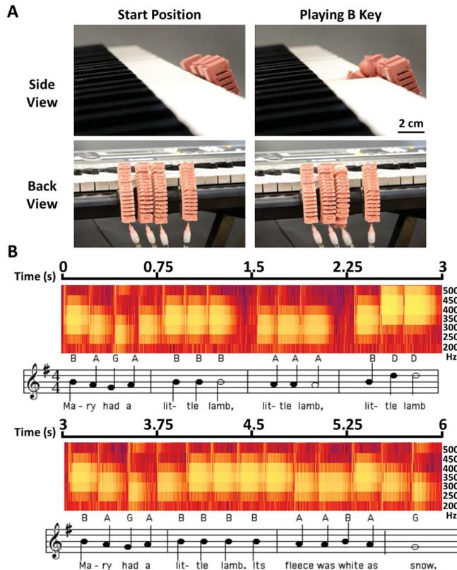
**Figure 6.** Independent Output Control. A) Images from two views of four fPN actuators playing a tune on a digital keyboard. Video is available in the on-line supplemental information. Each fPN was actuated for 75 ms at 103 kPa (except for repeated notes, which were actuated for 50 ms) and vented for 150 ms. B) Spectrum analysis of the audio file for frequencies between 200 and 500 Hz.
