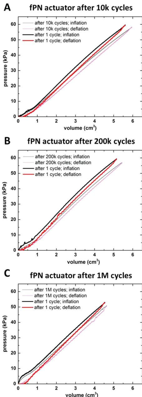
**Figure 4.** Fatigue test of fPN actuators. A–C) Pressure-volume hysteresis curves for fPN actuators before and after repeated pneumatic actuation. fPN actuators are made of Elastosil M4601 and paper and are hydraulically actuated to generate the PV curves.
